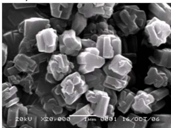
**Figure 4.** SEM image of Zn-Al-PAB prepared using zinc chloride and aluminium chloride at 20,000 magnification. The estimated crystallite was 300-500 nm.
