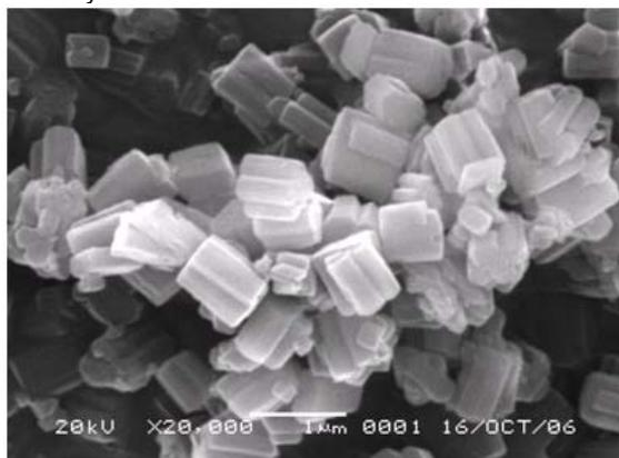
**Figure 5.** SEM image of Zn-Al-PAB prepared using zinc sulphate and aluminium sulphate at 20,000 magnification. The estimated crystallite was 700-900 nm.
