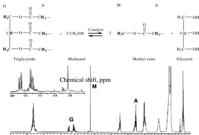
Fig. 1.  $^1\text{H}$  nuclear magnetic resonance (NMR) spectrum of a progressing transesterification reaction (spectrum recorded after 5 min reaction time at  $45^\circ\text{C}$ ). The letters **A**, **G**, and **M** denote the a-CH<sub>2</sub>, glyceridic, and methyl ester protons, respectively
