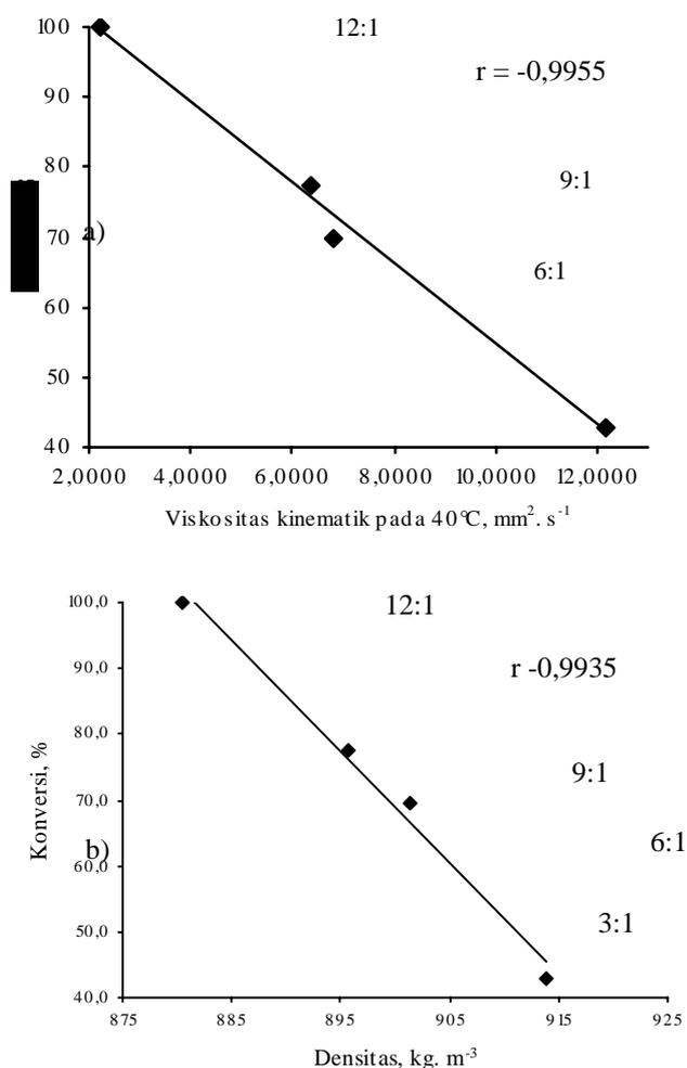
Fig. 3. The correlation of percentage of biodiesel conversion with physical properties: a) Kinematics viscosity at 40 °C; b). Density at 15°C biodiesel, in different methanol/oil molar ratio
